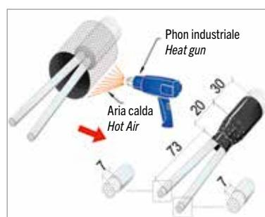
Position the TRDP6-B heat-shrink sheath as indicated and seal with the heat gun.
